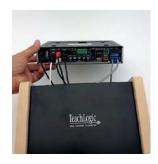
8. Plug in speaker connectors, sensor cable, power cable and auxiliary cables.
