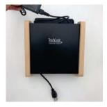
4. Place the amplifier power supply into the cabinet. Route plug through bottom hole.
