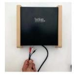
6. If external, route auxiliary cables (not provided) up through bottom.
